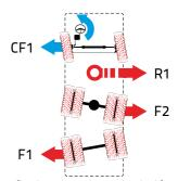
The conflict between the rear axles' forces F1 and F2 is transferred to the frame and results in the force R1. The resulting force R1 must be countered with the force CF1 by turning to the left.
